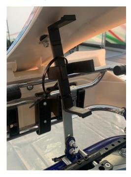
2) Place the battery in the housing and lock it with the supplied red tape.
