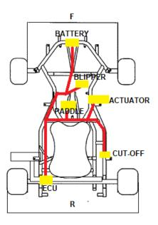
3) It is possible to cut and then insulate with electrical tape the cable parts not used for the go-kart by referring to the details in the electrical diagram attached (PERFORM THIS OPERATION WITHOUT POWER SUPPLY!);
