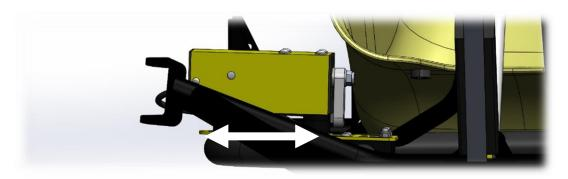
4) Lengthen the gear tie rod using the extension kit included in the kit;
